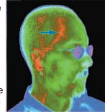
● The patented Arterial Heat Balance system computes the correct temperature by mathematically replacing the temperature that the blood lost in its short journey from the heart to the forehead.
